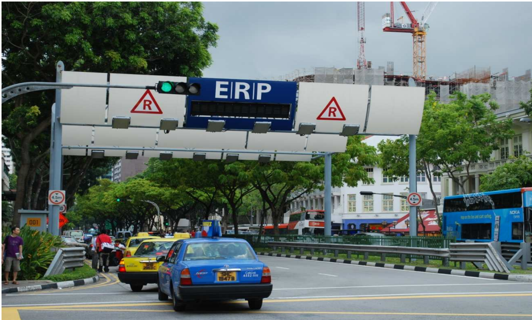
Caption: Singapore's Electronic Road Pricing system is highly dynamic and changes according to actual demand in a corridor. This is one of the various measures implemented by the city to manage congestion. Photo by Carlos Felipe Pardo.
